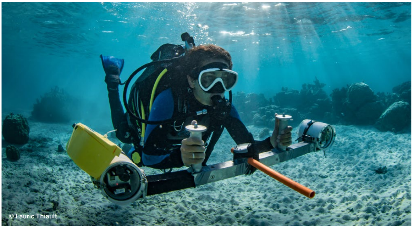
Figure 7. Example of a stereo video camera system for recording video to measure biodiversity and length.
